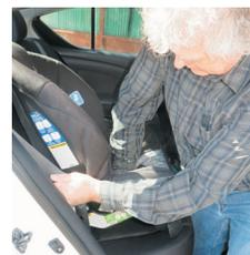
When tightening the belt, push the car seat down and into the vehicle upholstery. The seat should not move more than 2.5 cm (1 in.) toward the front of the vehicle, or directly side-to-side where the belt is attached. Rear-facing, it is acceptable (and normal) to be able to lift the seat toward the rear of the car or pivot it side-to-side.
